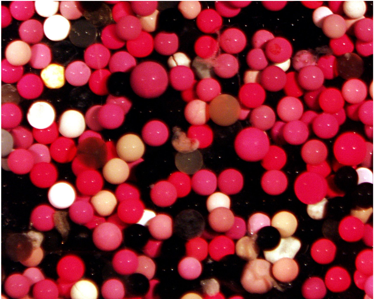
Figure 38. Plastic spheres found at the Formosa Discharge station FD in the HRI study. Spheres are about 0.5 mm in diameter.
